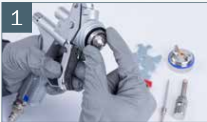
Assembly of the fluid tip
