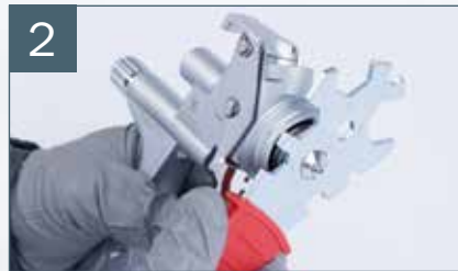
Hand-tighten fluid tip with universal spanner
