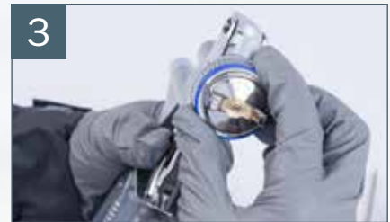
Assembly of the air cap
