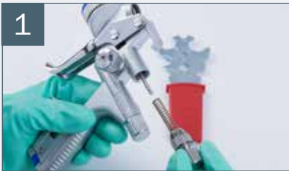
1 Removing the paint needle
