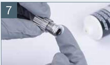
Lubricate* thread of material flow control screw
