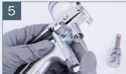
Assembly of the paint needle
