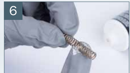
Lubricate* and insert paint needle spring
