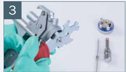
3 Unscrewing the fluid tip with the ring spanner integrated in the universal spanner.
